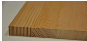
Random end grain patterns reduces cupping
