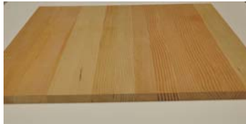
Random end grain patterns reduces cupping
